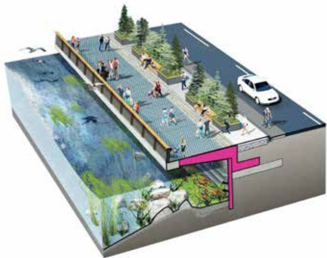
Figure 19: Illustration of the sea wall's ecological design (Seattle Department of Transportation 2016)
