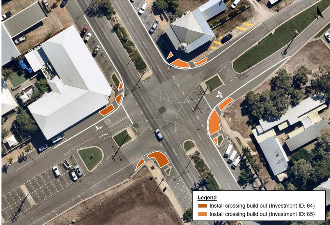
Figure 5.2: Concept Design of the Crossing Build Out Installation at the Dalrymple Street / Herbert Street Intersection
