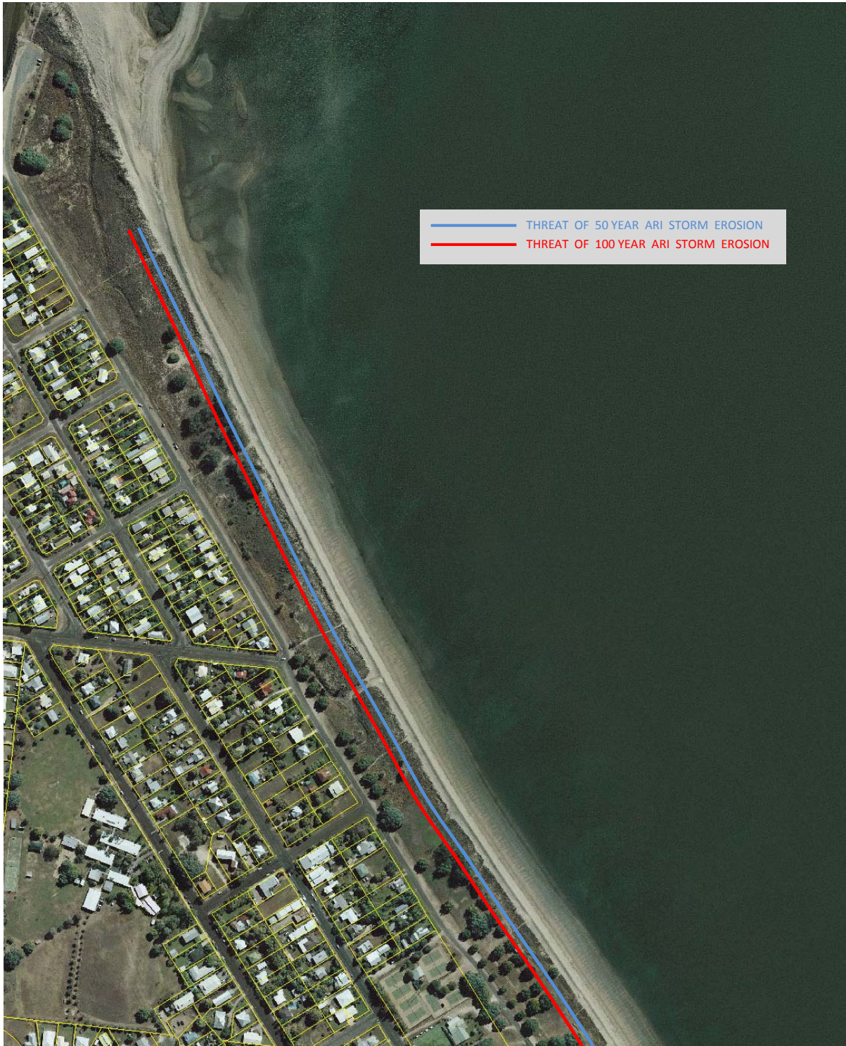
Figure 3.19 : Present-day Erosion Threat to the Foreshore of Queens Beach North
