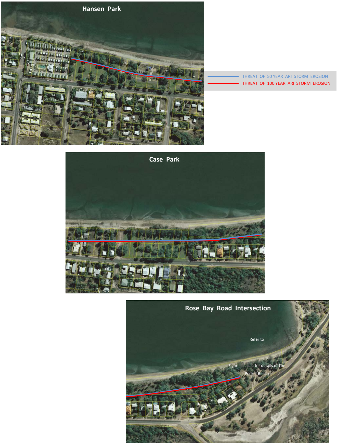
Figure 3.17 : Present-day Erosion Threat to the Foreshore of Queens Beach South
