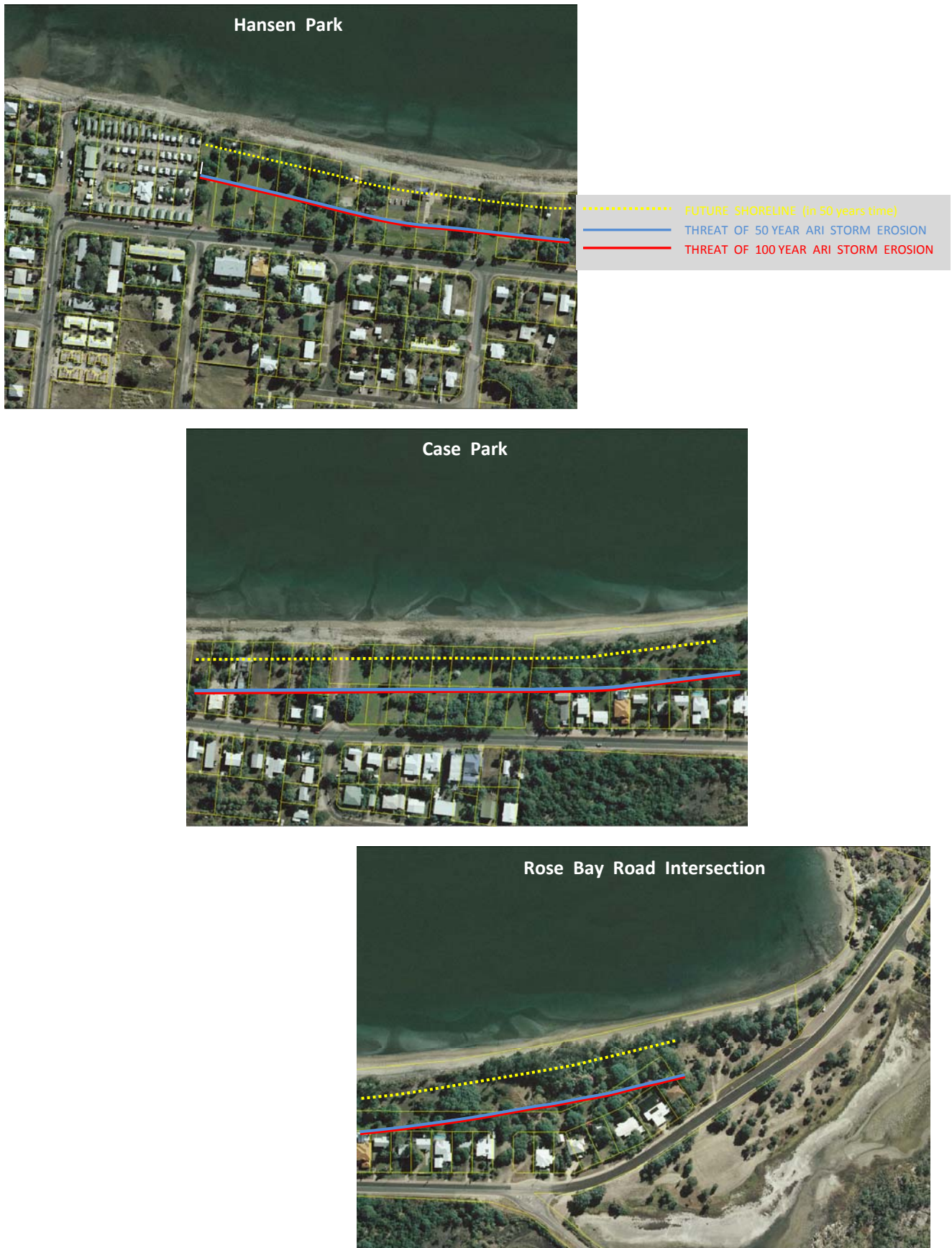
Figure 3.20 : Future Erosion Threat to the Foreshore of Queens Beach South
