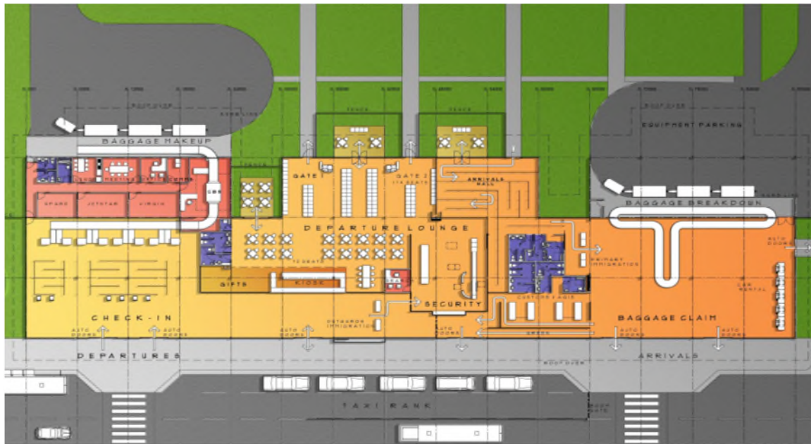
Figure 14: International configuration of existing terminal
