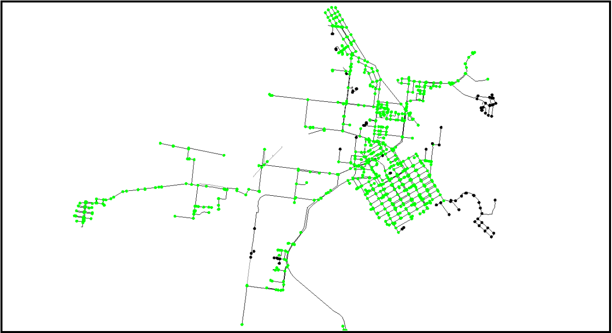
Figure 28 2014 Peak Hour Fire Flow Compliance – Bowen
